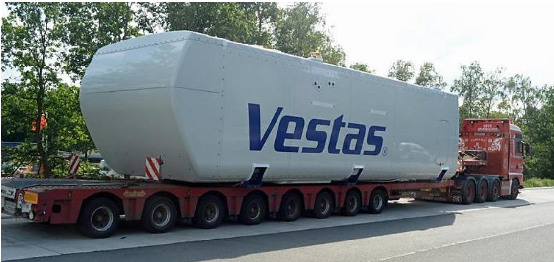
Figure 2.24: Example of a nacelle being transported (Source: Google Images, 2022)
