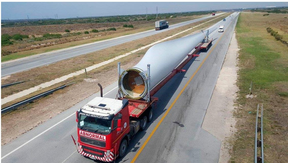
Figure 2.23: Example of a wind turbine blade being transported on an extendible trailer (Source: Google Images, 2022)
