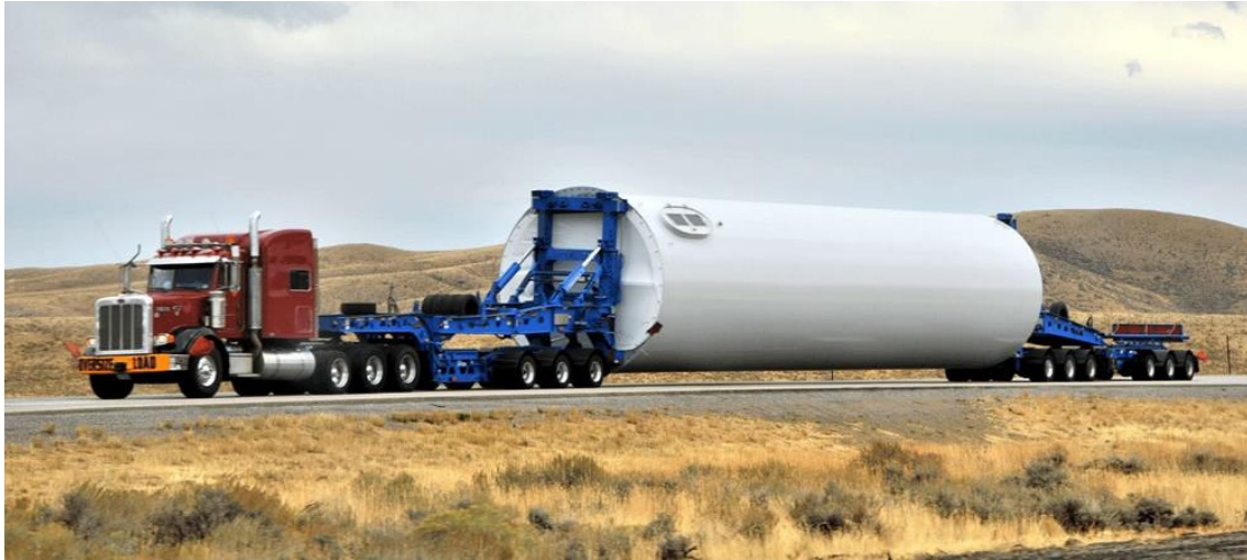
Figure 2.22: Example of a tower section being transported (Source: Google Images, 2022)
