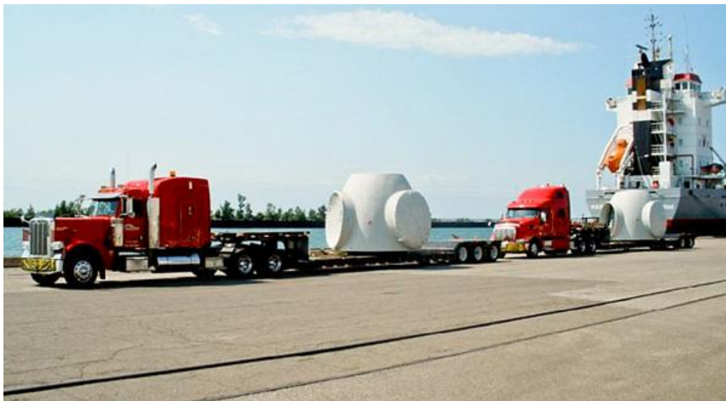
Figure 2.25: Example of a hub and rotary units being transported (Source: Google Images, 2022)
