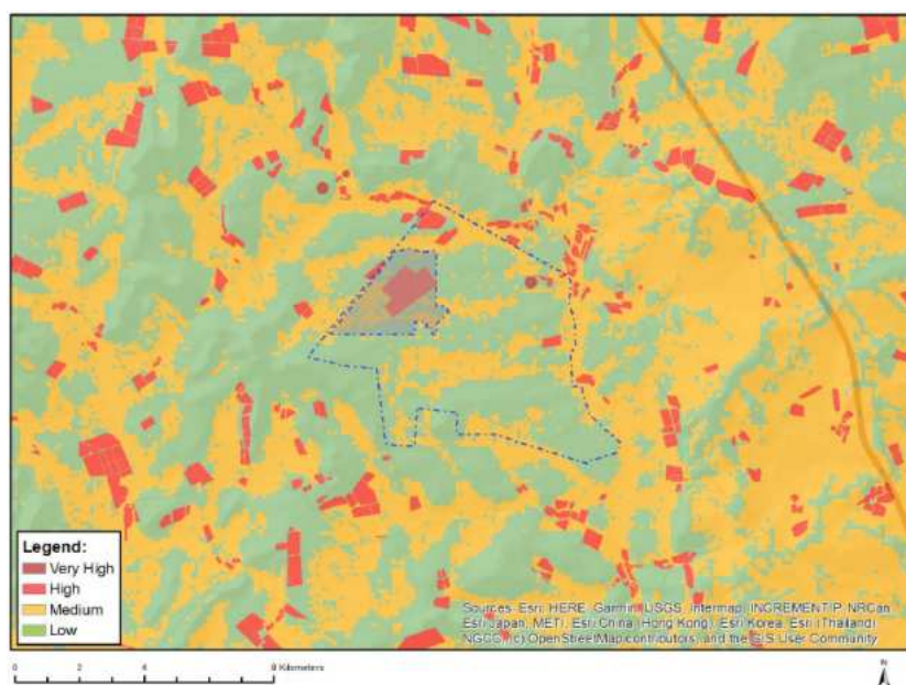
Figure 3.7: Agricultural sensitivity of the study area and project footprint for the PV facility and associated infrastructure overlaid on agricultural sensitivity based on the Screening Tool (Source: Screening Tool, 2024).
