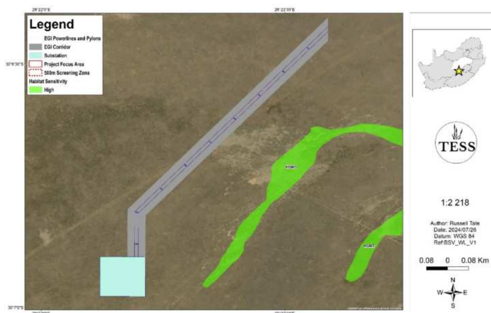
Figure 3.17: Layout and sensitivity map for the Aol and the proposed switching station and power line forming the EGI. On this map, seep wetlands shown in green are assigned High sensitivity (Tate Environmental Specialist Services, 2024).
